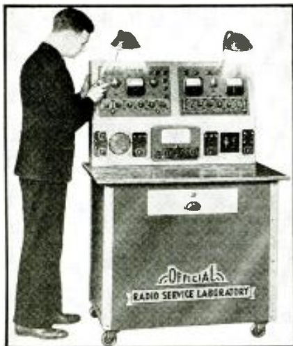
The "service shop on wheels," mentioned as a possibility in the June, 1936, issue of Radio-Craft is a reality. This unit combines: 1—vibrator analyzer; 2—receiver servicer; 3—R.F. oscillator; 4—universal speaker; 5—"B" supply unit; 6—multi-range antenna; 7—master control switch. (Write for additional data—ask for No. 1254)
